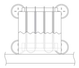
Do not cut or shorten the Hott-Wire® Cable Heating Element. Do not damage or subject the Hott-Wire® Heating Element to mechanical or shear stress from improper paver placement
