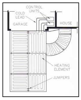
Sample Driveway and sidewalk layout for two Hott-Wire® MI Cable snow melting sets. Note that jumpers extend the Hott-Wire® heating element through all joints and marks.
