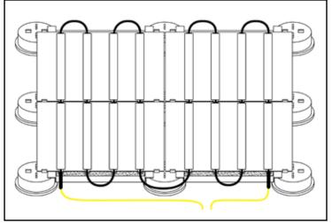
While laying the cable, small strips of tape can be used to temporarily hold the cable in place allowing for length adjustments at turns to accomodate the fixed length cable to be installed fully in the pans and transition cold connections out of the pan as previously referenced. Once the cable is completely laid out, the aluminum tape should fully cover the Hott-Wire® that is positioned in the pans to secure it for paver installation.
